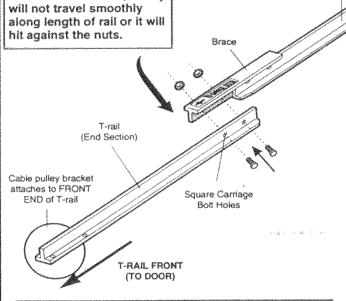
• Position the cable pulley bracket on the front end of the T-rail as shown. Fasten securely with the hardware.
